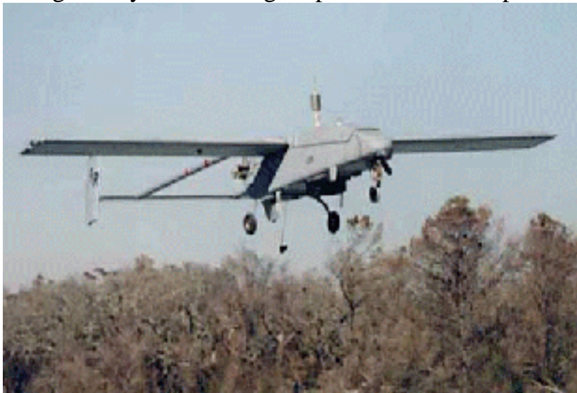
COBRA is a UAV-based optical sensor system used by the Marines to detect minefields
