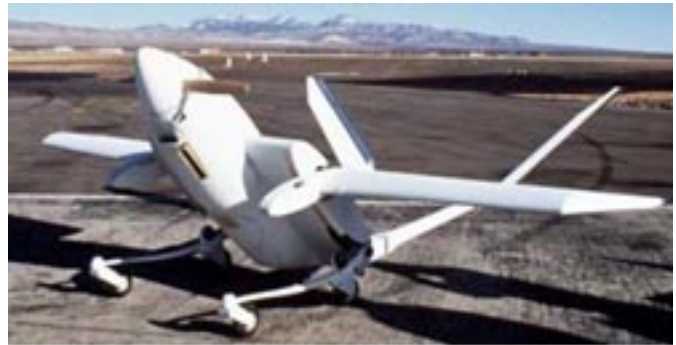
The Freewing incorporates a constant aspect free-floating wing and thrust vectoring with only three moving parts
