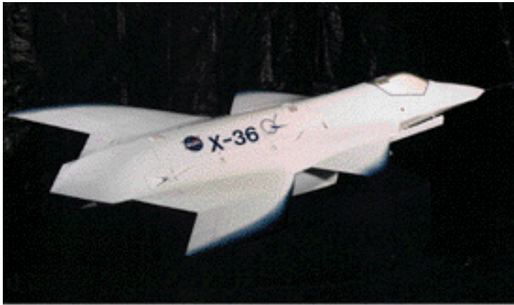
The X-36 is a small, remotely-piloted jet designed to fly without the traditional tail surfaces common on most aircraft
