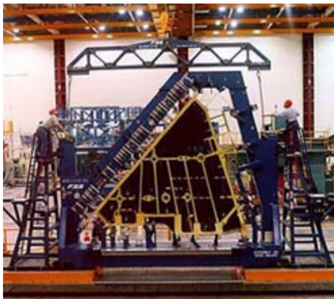
The first wing for the first F-22 is moved into position for high-precision drilling at the Boeing plant in Seattle
