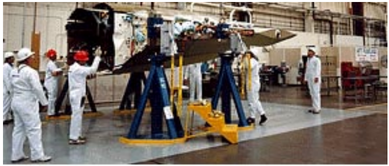
Boeing crane operators load the aft fuselage for the first F-22 fighter into a shipping container at the Boeing Development Center in Seattle for delivery to Lockheed Martin in Marietta, Ga.
